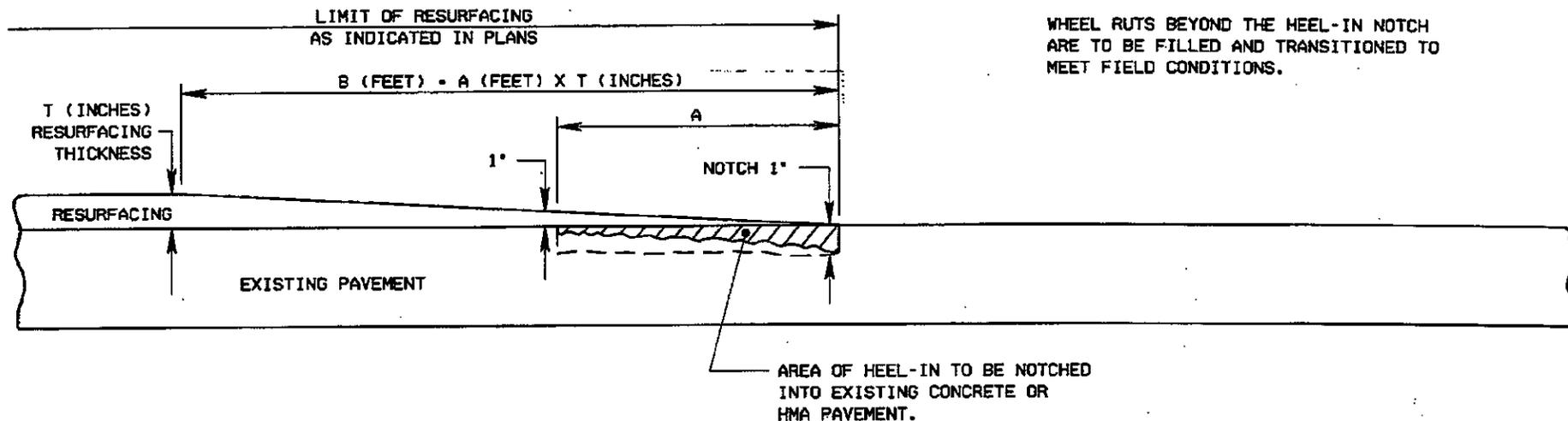
WHEEL RUTS BEYOND THE HEEL-IN NOTCH ARE TO BE FILLED AND TRANSITIONED TO MEET FIELD CONDITIONS.
